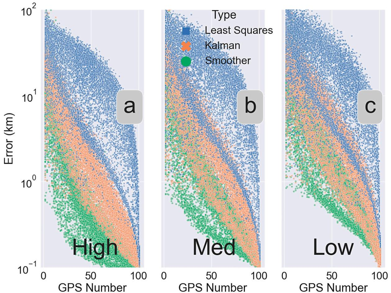
FIG. 6. Trajectory error for numerical simulation for Kalman smoother (green circle), Kalman filter (orange  $\times$ ), and least squares (blue squares) algorithm for varying percentage of GPS positioning. The  $s$  value [Eq. (1)] is equal to (a) 10%—high signal-to-noise case; (b) 30%—medium signal-to-noise case; and (c) 70% of mean flow—low signal-to-noise case.
